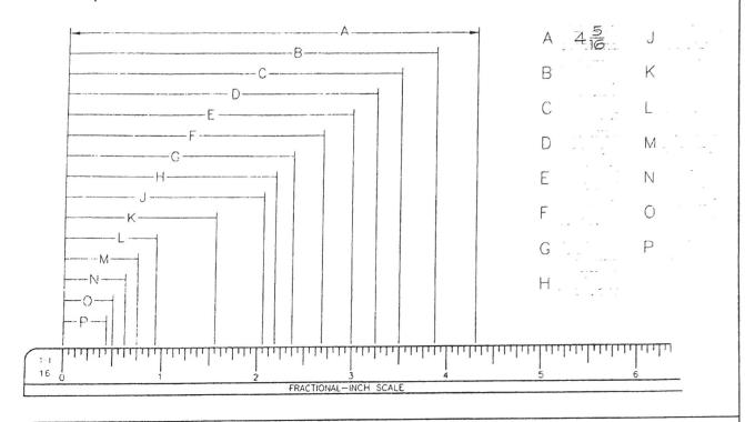
**Problem 3-7:** Using a full-size fractional-inch scale, measure each of the lettered lines in the figure below. Record the length of each in its corresponding space at the right. Measure all lines to the nearest 16th of an inch.
