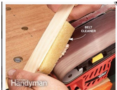
A belt cleaner cleans the sawdust out of an abrasive pad.
